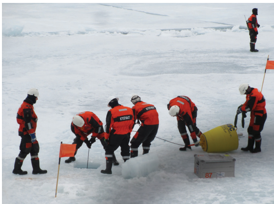
Deployment of an integrated ocean acoustic ice station in the Fram Strait under the UNDER-ICE project.
